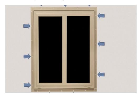
Re-check for plumb, level and square prior to nailing the jambs.
