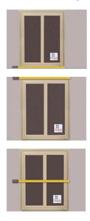
After this has been done, place a temporary 2" roofing nail at the mid-point of the head,
