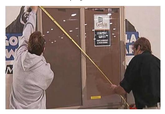
To check for bowing you should measure the sill, head and at the mid-point widths.
