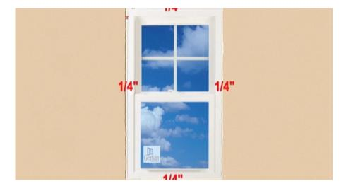
Double-check the size of your rough openings on the inside and the outside of the opening by measuring the edges and the mid points of your rough opening. The required rough opening size must be maintained at every point within the rough opening.
